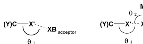
Fig. 5. Expected geometries for the approach of a neutral organic XB acceptor (left) and a metal-bound halogen atom (right) to an electrophilic C-bound halogen atom.
